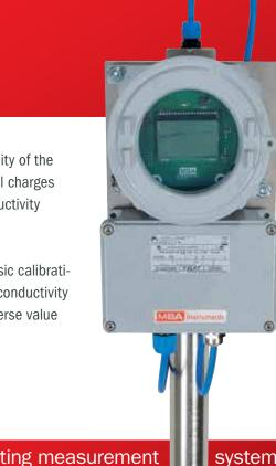
Conductivity: 5 to 2,000 pS/m, expandable to 5 to 10,000 pS/m, with simultaneous temperature measurement in °C Display unit MLA1000-A: 🕢 II 2(1)G Ex de [ia Ga] IIB T4 Gb
